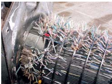
Filter blocked by cotton buds (Nicki Souter)
